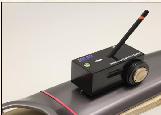
Pencil Hardness Test
